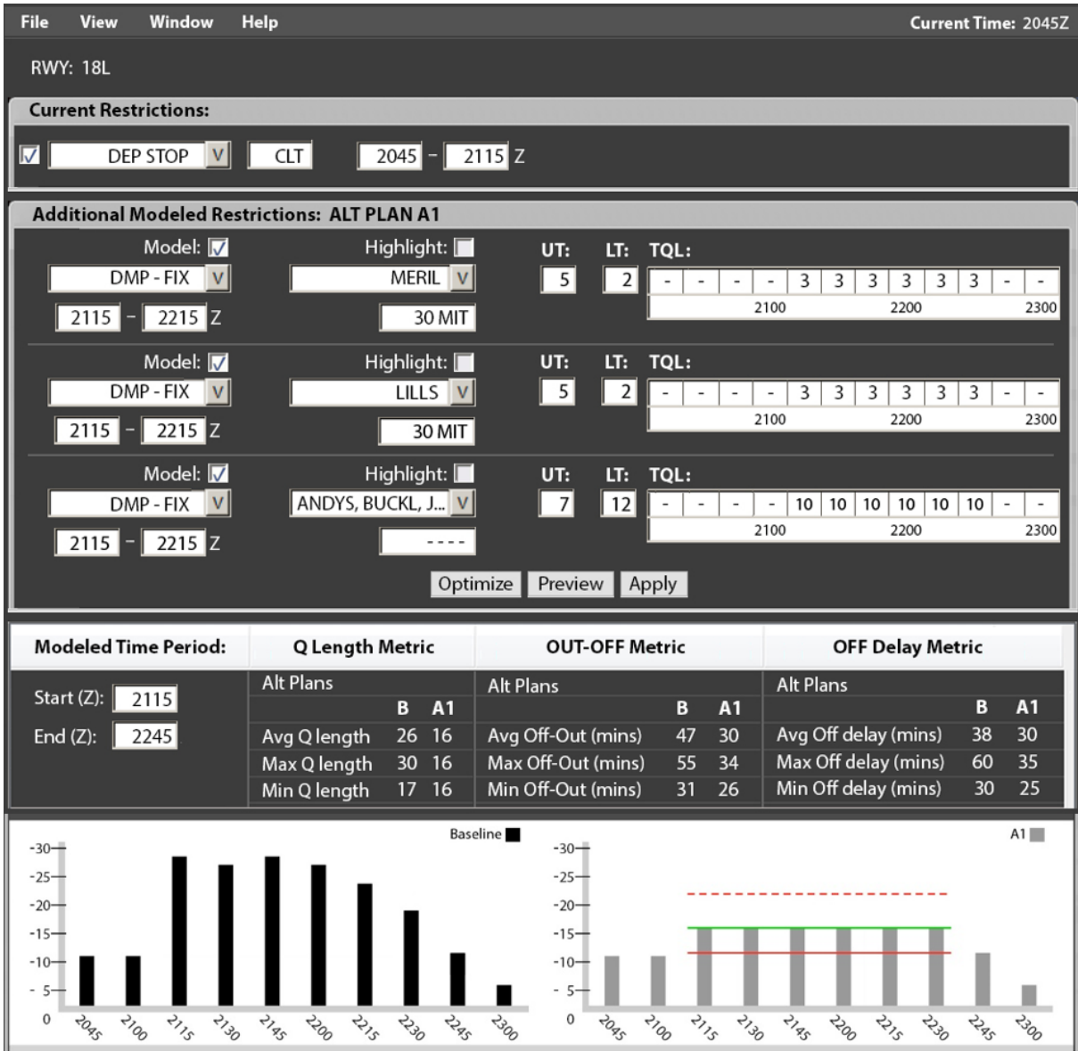
Figure 6-5. Bar Charts Comparing Predicted Queue Lengths for 18L With and Without the Implementation of the Modeled Categorical DMPs in Combination With the Implemented Departure Stop.
